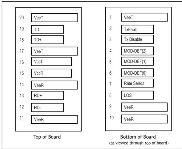
Pin Description and Plug-in Sequence<sup>1</sup> (1-Grd, 2-Power, 3-Signal)
