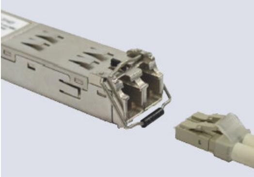
The OFD2300 transceiver module operates at a wavelength of 850 nm and at 1.25 Gb/s for Gigabit Ethernet 1000BASE-SX and 1x Fiber Channel applications.
