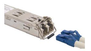
The OFD2400 transceiver module operates at a wavelength of 850 nm and at 2.1 Gb/s for 1x/2x Fiber Channel and Gigabit Ethernet 1000BASE-SX applications.
