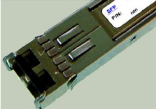
The OFD3357 transceiver module operates at a wavelength of 1550 nm and at 1.25 Gb/s for Gigabit Ethernet 1000BASE-ZX and 1x Fiber Channel applications.
