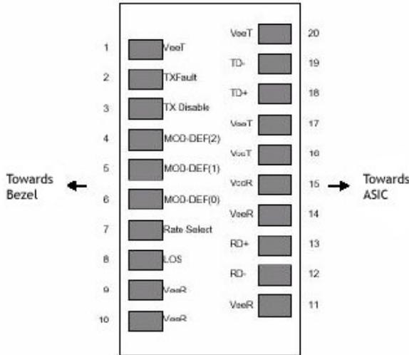
Figure 2. Diagram of Host Board Connector Block Pin
