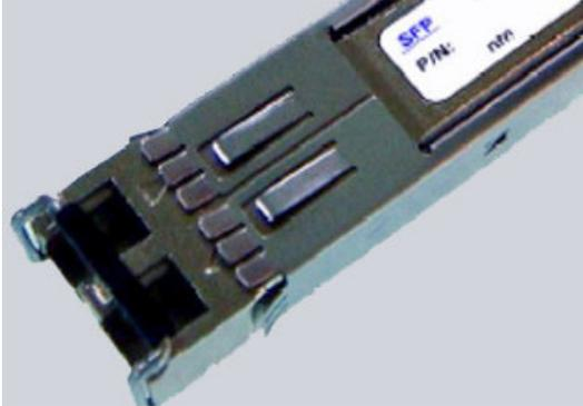
The OFP3456 transceiver module operates at a wavelength of 1550 nm and at 2.5 Gb/s for OC-48/STM-16 intermediate reach applications.
