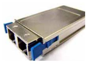
The OGB3357 transceiver module operates a wavelength of 1550 nm and at 1.25 Gb/s for 1000BASE-ZX.
