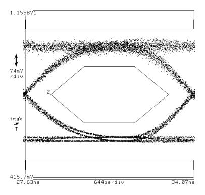
Bessel-Thomson filtered typical output waveform.
