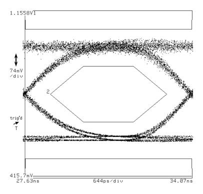
Bessel-Thomson filtered typical output waveform.
