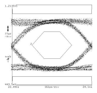
Bessel-Thomson filtered typical output waveform.
