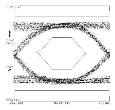
Bessel-Thomson filtered typical output waveform.
