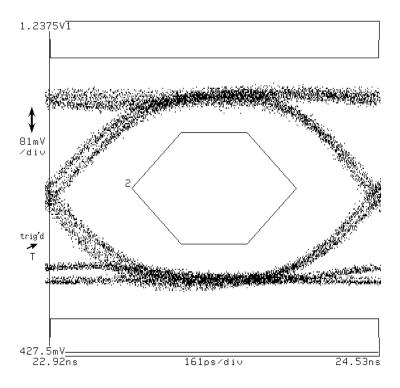
Bessel-Thomson filtered typical output waveform.
