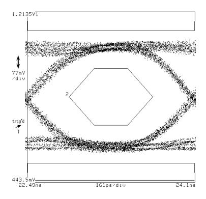
Bessel-Thomson filtered typical output waveform.
