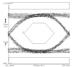
Bessel-Thomson filtered typical output waveform.
