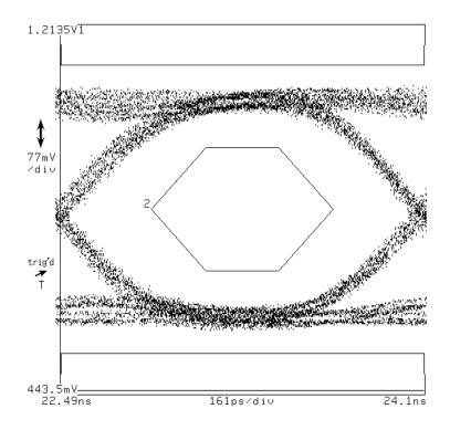
Bessel-Thomson filtered typical output waveform.
